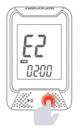
5) Hold from than 2 seconds to exit the setting mode and save
